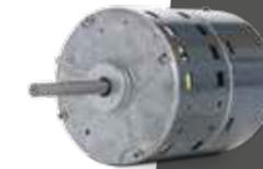
8. Blower Motor: A variable speed ECM motor runs at only the speed needed for maximum efficiency and savings. Other choices include a standard PSC or high efficiency 5-Speed ECM blower motor for comfort and quiet operation.
