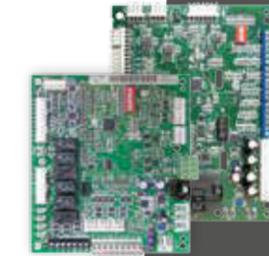
7. Aurora Controls: The powerful Aurora Base Control (ABC) offers two way communication between components, advanced operating logic and robust troubleshooting capabilities. The Aurora Expansion Board (AXB) adds support for true energy monitoring, extended hot water generation control and more. AXB also expands communication to include the internet, the smart grid, home automation networks and our IntelliZone™ zoning system.
